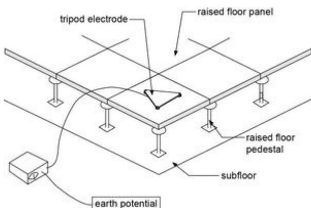
Tripod electrode: Aluminium panel with rubber feet
